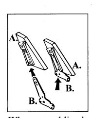
When assembling back to arms, place Bracket B into Sleeve A and press top of back down firmly to lock the retaining clip into place.
