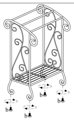
Tighten Adjustable Levelers (b) to the bottom of Side Frames (A) & (B). Note: Please adjust Levelers (b) if this unit is not stable.
