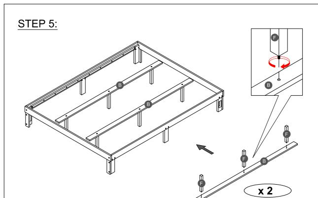
Assembling leg support (F) with lower support slat (B) later rotate, Move support slat inside Queen bed.
