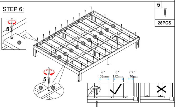
**NOTE:** Please make sure the bed slats close to the side rail before locking the screws to avoid breakage. This step is required for both the left and right sides. Moreover, please do not lock the screws of the bed slats at the outermost edge to avoid damaging.
