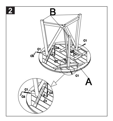
Step 2: put the legs to the table top (A) as shown on the picture. Use the Allen bolts (C1) to fit all the legs to the table top (A) as shown on the picture by using the Allen key (C4) and Wrench (C5).
