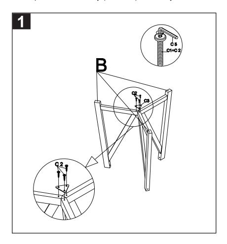
Step1: assemble the 3 legs (B) together with the triangle part (C3) as shown on the picture by using the Allen screws (C2) and tighten all with the Allen key (C5).
