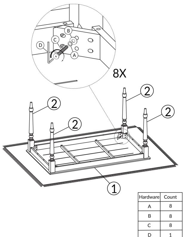
TIGHTEN BOLT COMPLETELY.
