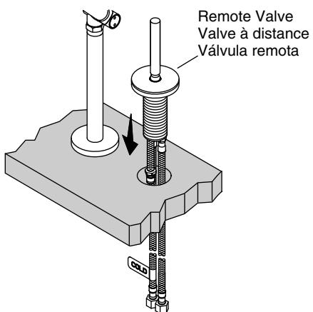
**8** Position the remote valve with the cold water supply on the left **AND** the spout connection toward the front of the sink.
