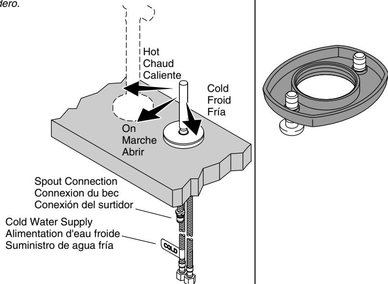
**9** Partially thread the screws into the ring.
