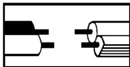
\*Note: When parallel wire ( SPT I & SPT II ) is used. The neutral wire is square shaped and ridged and the hot wire will be round in shape and smooth. ( See Illustration on left. )
