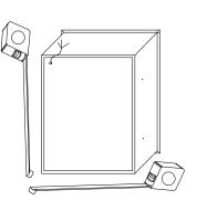
2. Measure the width and height of the back side of the cabinet.
