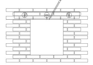
3. According to No.2, Draw a leveled rectangle on the wall with track level bar, that is about 1/5 inch larger than the cabinet recess in both width and height to make sure the fit not too tight. Make a hole that the depth is larger than 4.6 inch.
