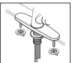
(3b) Thread and tighten both mounting nuts to mounting bolts from underneath the sink to secure faucet on the sink.
