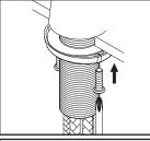
(2c) Thread locknut onto the faucet shank from underneath the sink. Position faucet to desired location from the top and handtighten locknut till it won't go further. Thread both screws on locknut and tighten screws on locknut with the help of a Phillips head screwdriver to secure faucet. (Note: Do not overtighten.)
