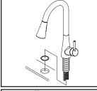
(2a) For 1-Hole Installation:- Ensure there is a washer under the faucet. Place the faucet in position on the sink.
