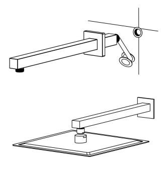
Before installing the faucet, please be sure to remove sundries and sludge from the water pipe to prevent sundries from blocking the faucet.
