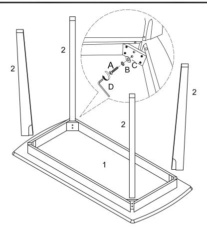
Insert the legs (2) into top panel (1), use wrench (D) to secure it with bolt (A), spring washer (B) and washer (C).
