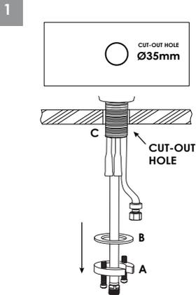
Ensure there is a  $\varnothing 35\text{mm}$  through-hole on the kitchen counter. Remove the mounting nut (A) and washer (B) from the threaded shroud (C).
