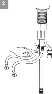
Connect braided supply hoses to faucet female outlets, secure firmly by hand until hose is snug to pipe.
