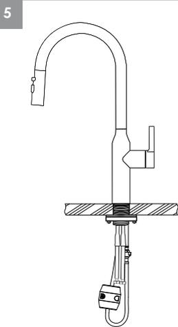
Secure weight on lowest vertical point on pull-out hose side. (not on quick connect side).
