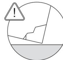
**Caution:** The most fragile parts of tempered glass panels are the corners. Therefore, it is critical you have the rubber blocks in place so the glass never touches the tile surface you are installing onto. Please make sure the glass is always on cardboard packaging or rubber blocks while out of the packaging prior/during install. Rubber block is provided in your hardware pack however you can use wood, cardboard or other rubber products to protect against breakage.
