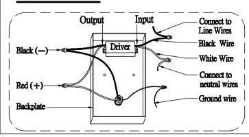
The fixture is designed to dim with a standard Triac forward phase dimmer. Dimming levels will vary by dimmer.
