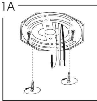
Carefully pull house wires through opening in center of mounting plate. With mounting plate threads facing outward, screw mounting plate into junction box using outlet box screws.
