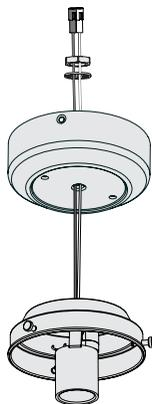
Feed the wires through the center hole in the switch housing, the washer, and the nut. Then install the switch housing by twisting clockwise onto the threaded rod. Install the washer and nut onto threaded rod and tighten securely.
