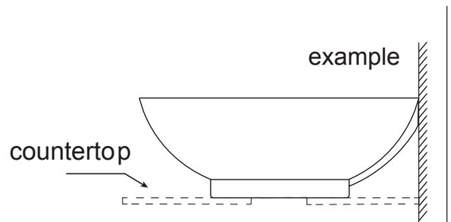
**Step 3:** Place a generous portion of plumbers' putty under drain cap and insert whole drain body inside the bowl and through the countertop
