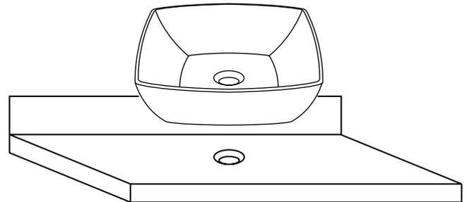
**Step 3:** Place a generous portion of plumbers' putty under drain cap and insert whole drain body inside the bowl and through the countertop.
