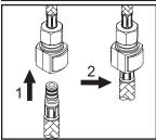
(4) Insert spray head hose into end of quick connect adapter on the outlet hose, push until a "click" is heard. Pull down to test engagement.
