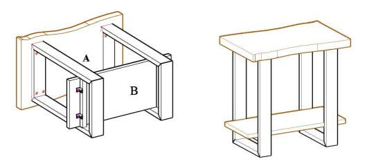
TIGHTEN ALL BOLTS FIRMLY AT THIS TIME USING ALLEN KEY (F). SET 1 SHELF END TABLE UPRIGHT.
