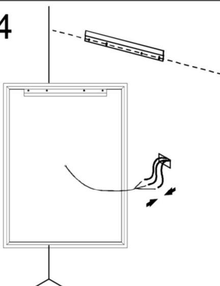
Connect to 120 VAC, 60Hz power supply.
