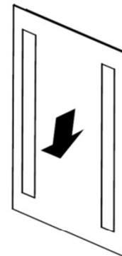
Press the mirror down slightly and make sure the brackets fit properly.
