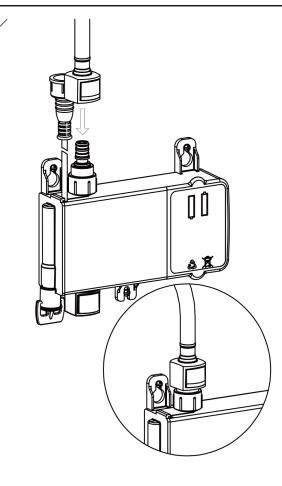
Connect the outlet hose to the control box with our innovative "quick connection".
