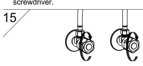
When installation steps 1-14 are completed, turn the hot & cold water inlets back on.
