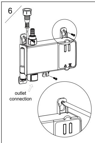
Mount the control box under the sink by a cross screwdriver according to the referential dimension, leaving some adjusting space.
