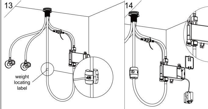
Install the counterweight on the pulldown hose at the marked position (the weight should be placed between this mark), and fix them by a cross screwdriver.
