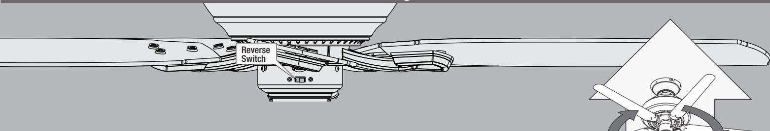
Ceiling fans work in two directions: downdraft (counterclockwise rotation) and updraft (clockwise rotation). To change the direction of air flow, turn the fan off and let it come to a complete stop. Slide the reversing switch to the opposite position. Restart the fan.
