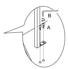
Attach part (3,4,5) to part 1 using bolt (A) with hex key (B).
