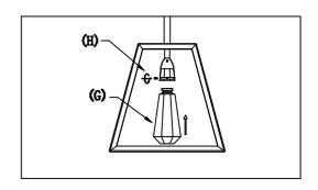
Step 2: Attach crystal (G) to fixture using Allen screws (H) provided.
