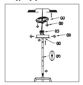
Step 1: Run wire through stems (F) and combine stem lengths to meet desired mounting height. Remove mounting bracket (A) from fixture and install to electrical box. Wire fixture (C) to wires in outlet box. Green wire is Ground wire. Attach the canopy (E) to the mounting bracket using screws (D) on the sides to secure.
