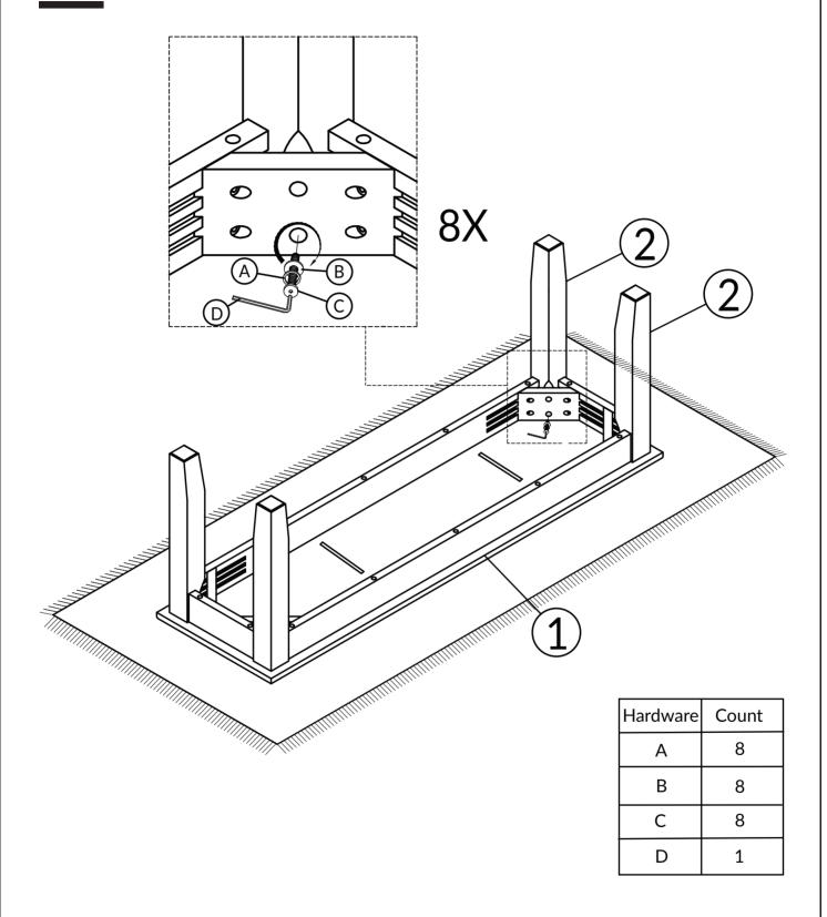
TIGHTEN BOLT COMPLETELY.
