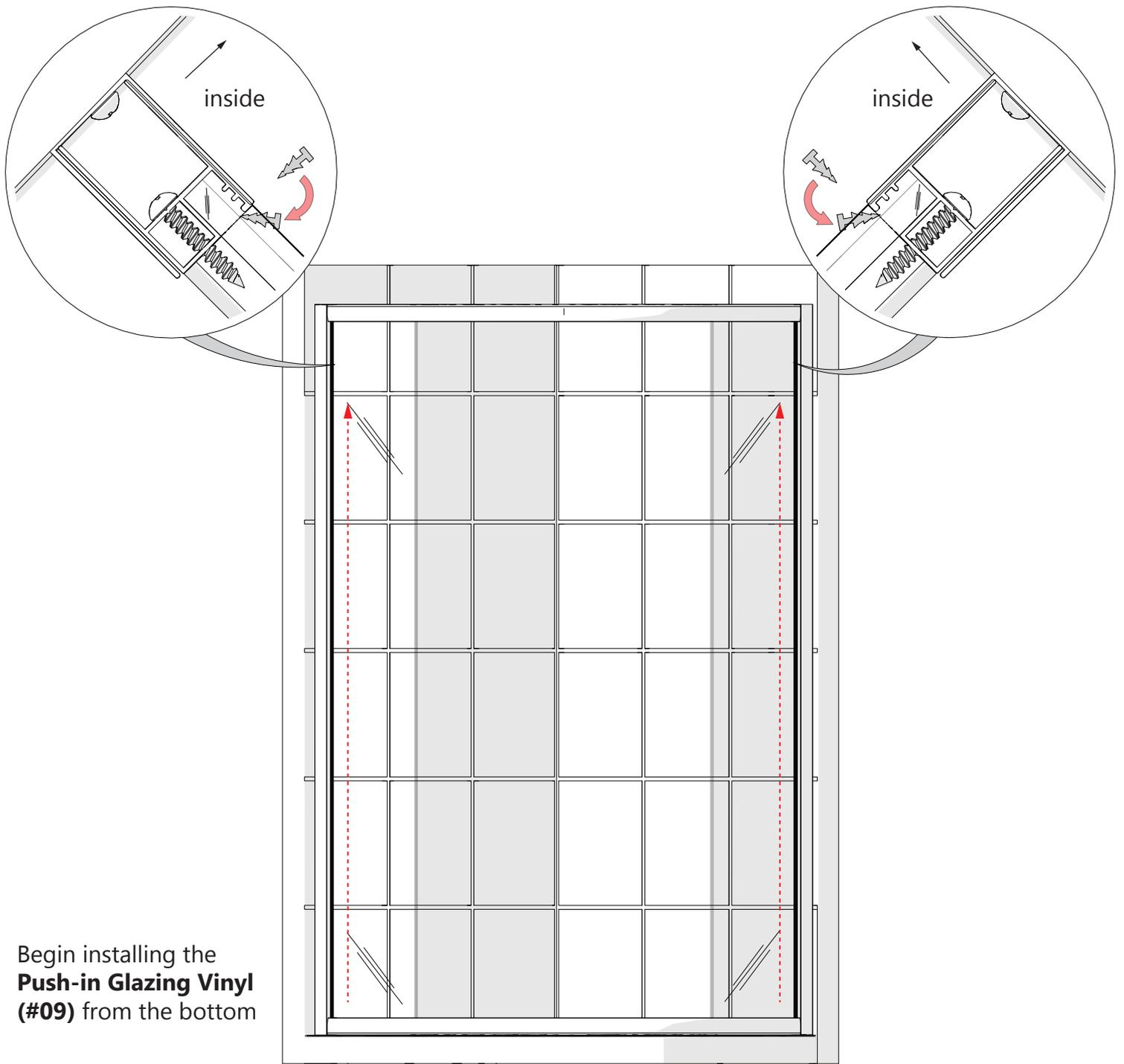
Begin installing the **Push-in Glazing Vinyl (#09)** from the bottom
