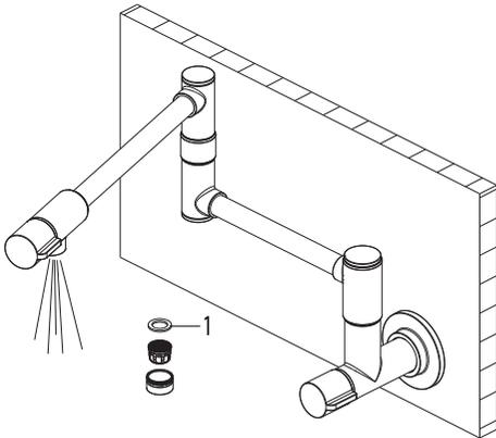
After the installation is complete, remove the aerator and housing by unscrewing it from the spout in a counterclockwise direction. Turn on the two handles to the right, turn on the water supply and allow water to run for at least one minute. This flushes away any debris that could cause damage to internal parts. Check for leaks. Reattach the aerator and housing. Do not lose the washer (1) in the aerator.
