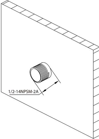
Install the supply piping so that the 1/2-14NPSM-2A threaded connection protrudes approximately 1/2-14NPSM-2A beyond the finished wall.
