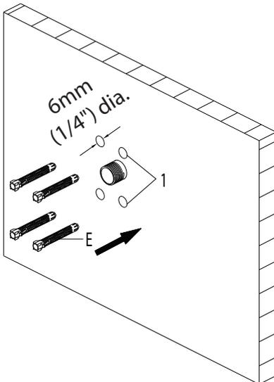
Insert the anchors (E) into the holes (1) and tap flush with the wall.
