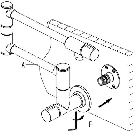
Rotate the faucet assembly (A) until the correct alignment is made (spout should be pointing straight down). Push the faucet body onto the quick connector over the two o-rings. The splines inside the faucet body should line up with the splines on the connector. Secure the faucet assembly (A) by tightening the bottom set screw (already pre-installed inside the faucet assembly) with the hex wrench (F).
