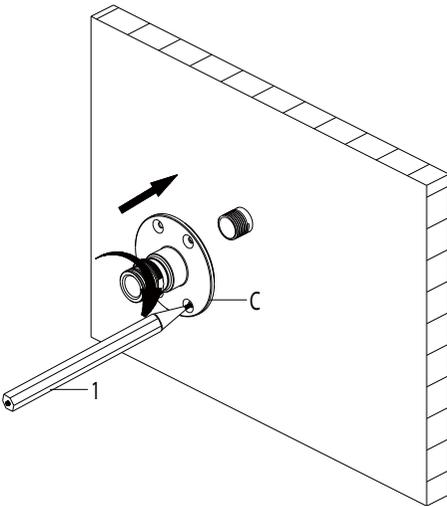
Install the seat (C) onto the finished wall. Screw the seat onto the supply piping and mark the locations for the support screws with a pencil (1).
