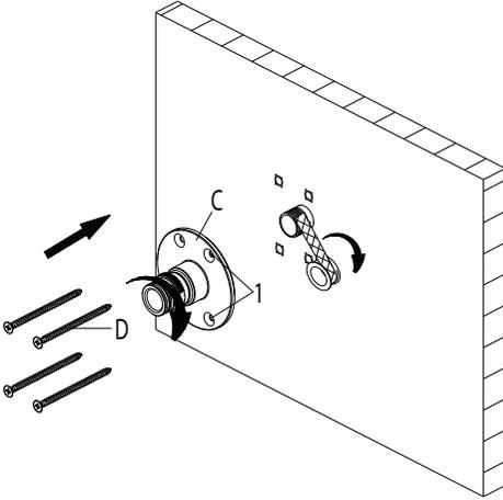
Apply pipe sealant tape to the threads of the supply pipe in a clockwise direction, as shown. Screw the seat (C) onto the supply piping and insert the screws (D) through the mounting bracket holes (1) and tighten until the seat (C) is flush with the wall. Do not over tighten.
