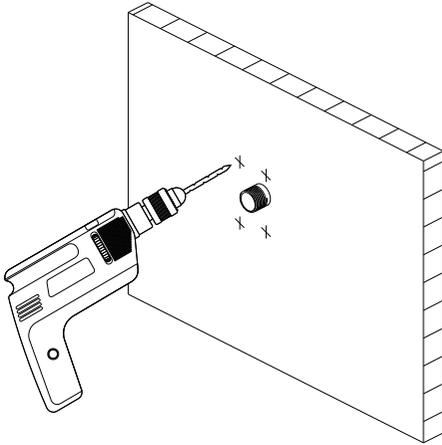
Remove the seat and drill four holes on the positions marked in step 2 using a 6mm (1/4 in.) diameter drill bit.
