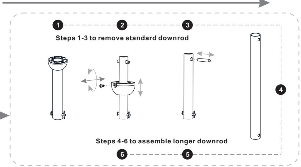
**3 Install Rod to Fixture Body**
