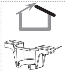
This fan cannot be used for the ceiling which angle is greater than 10 degree.
