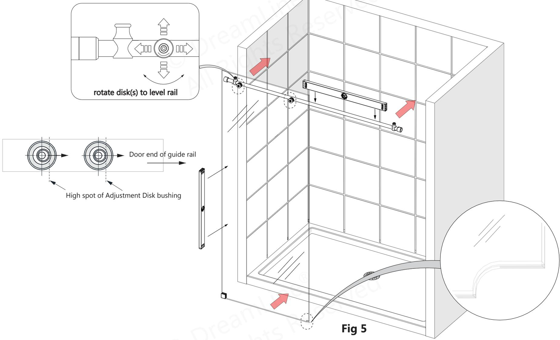
**NOTE** The **Panel Glass (#02)** must be installed to the **outside** of the **Top Guide Rail (#03)**.
