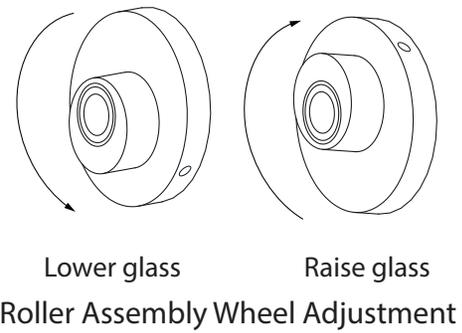
**TIP** Mark the location of the high spot on the outer surface of the adjustment disk with a felt tip pen to make adjustment easier to see.
