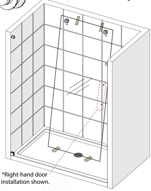
Before installing the **Panel Glass (#02)**, attach the two **Roller Assemblies (#04)** to the **Door Glass (#05)** with the wheels facing outside of the shower. Align the **safety set screw** towards the top for easier access. Then, take the **Door Glass (#05)** into the shower area and lean it against the wall with the handle holes on the correct side. Always use padding to protect the glass and shower surfaces.
