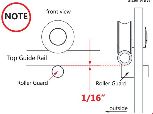
**!** Position the **Roller Guard (#29)** 1/16" below the rail. Hold the roller guard bolt with the **Allen Wrench (#11)** and tighten the interior post using a small allen wrench (**Fig 22.2\***)
