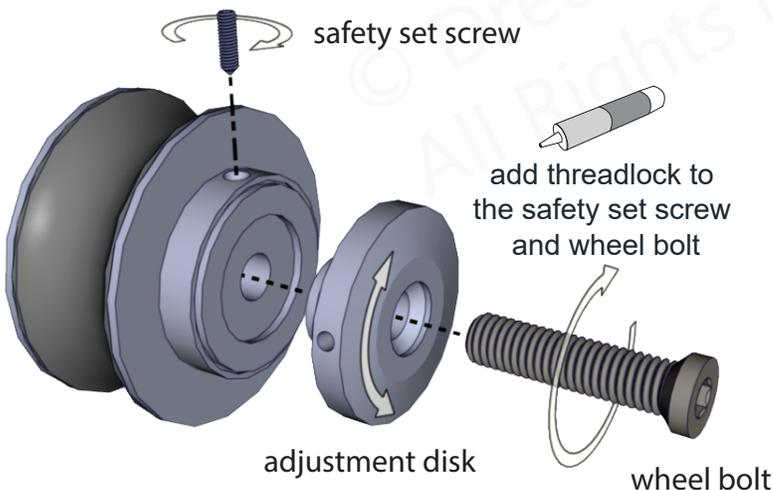
The provided Thread Lock will remain workable for approximately 10-15 minutes before drying.
