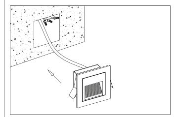
3. Install Light •Tuck wires into cut hole. Insert fixture into hole.
