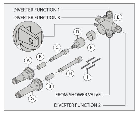
**Note:** For diverter valves purchased before November, 2016, retaining sleeve (F) must be inserted flush into diverter valve body (E) before installing cartridge (D).
