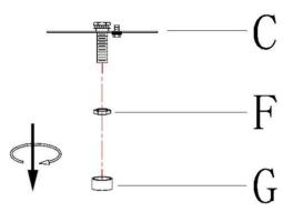
4 » Secure single bar (C) to the outlet box with mounting screws (B).
