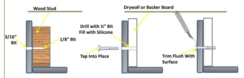
If the drilled holes go directly into a stud, switch to a 1/8" bit to drill the stud. To prevent water infiltration, fill the hole with silicone before installing screws.
