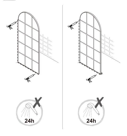
• Do not use the shower enclosure for at least 24 hours in order to allow the silicone sealant to cure fully.
