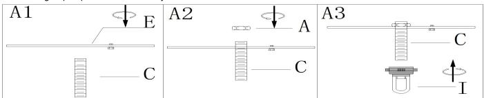
Step A1: Thread the single bar(E) over the nipple (C) a minimum of 6 mm (1/4"). At this point need note that: the side of single bar marked "GND" must face to the down.
