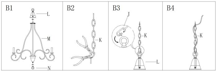
Step B1: Thread the upper trim (L)onto the fixture body (M) till tight .
