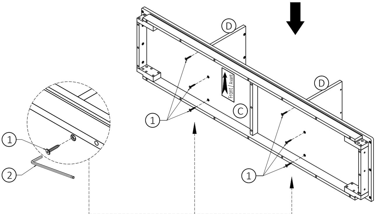
2. Use six Allen Key Screws (1) to attach Dividers (D) through guide holes from Bottom (C) to pre-drilled holes of Dividers (D).
