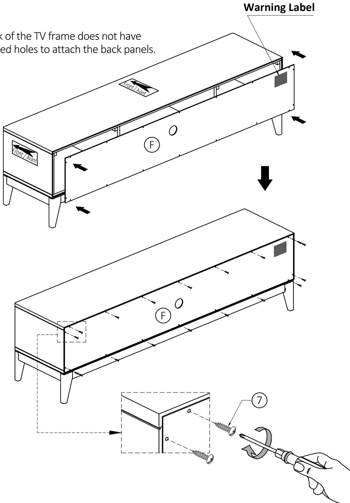
1. Attach the Back Panel (F) to back frame using Phillips Screws Round Head (7) through guide holes from Back Panel.
