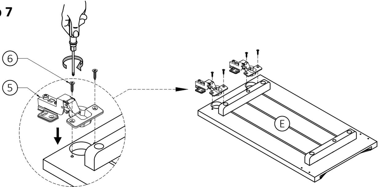
1. Attach Adjustable Hinges (5) to Doors (E) using Phillips Screws (6) into pre-drilled holes on Doors (E).
