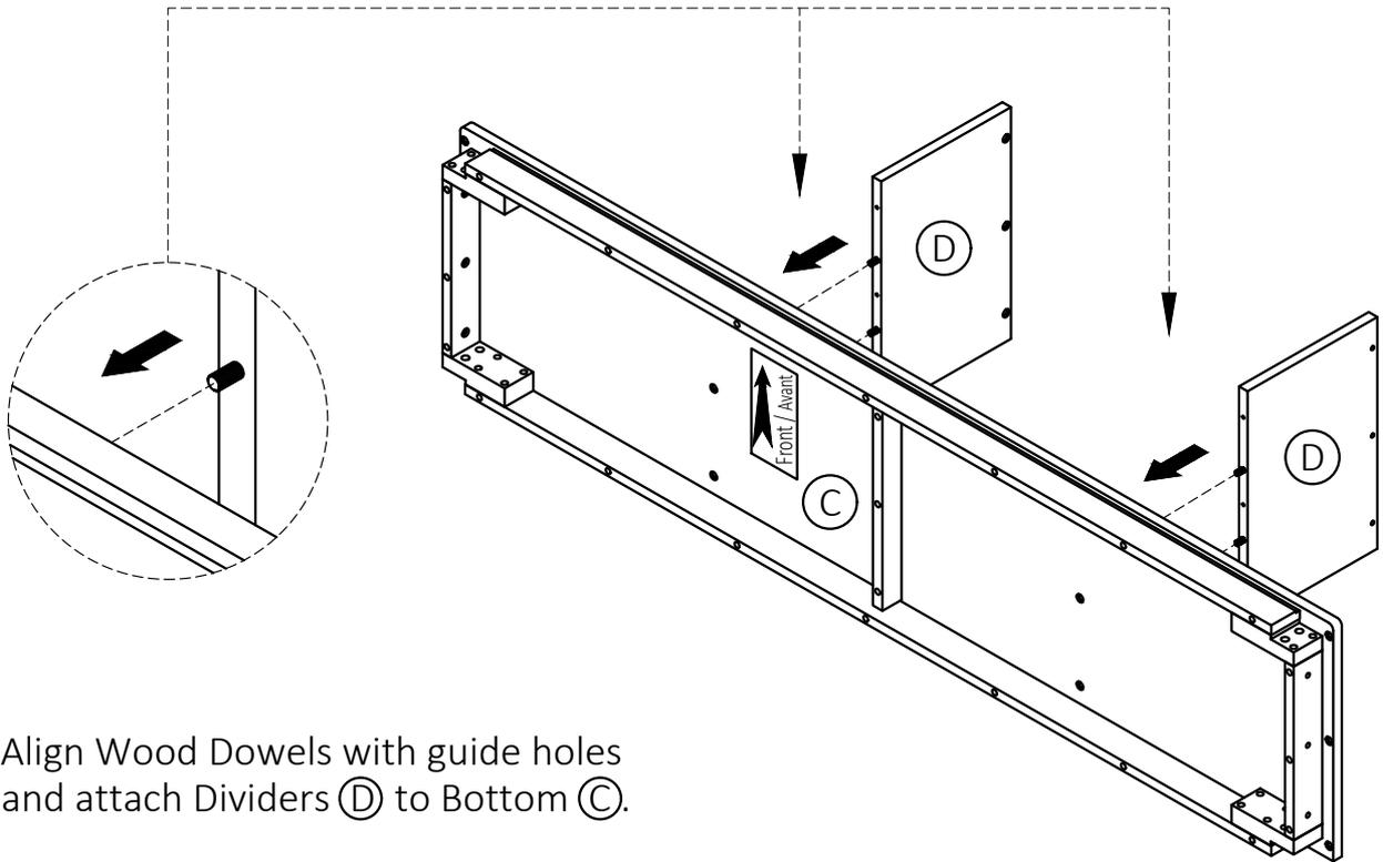
1. Align Wood Dowels with guide holes and attach Dividers (D) to Bottom (C).
