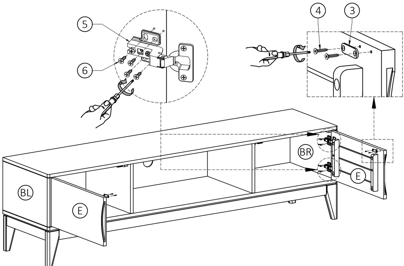
2. Attach Adjustable Hinges (5) on Doors (E) to parts (BL), (BR) using Phillips Screws (6) into pre-drilled holes on parts (BL), (BR).
