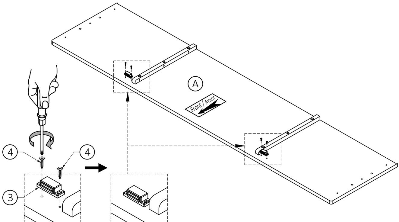
3. Attach Magnets (3) using Phillips Screws (4) into pre-drilled holes Top (A).
