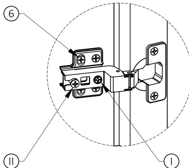
Tighten the Screw marked ② to fasten hinge. The door may need to be adjusted so that all the spaces between the door and the unit sides are equal.
