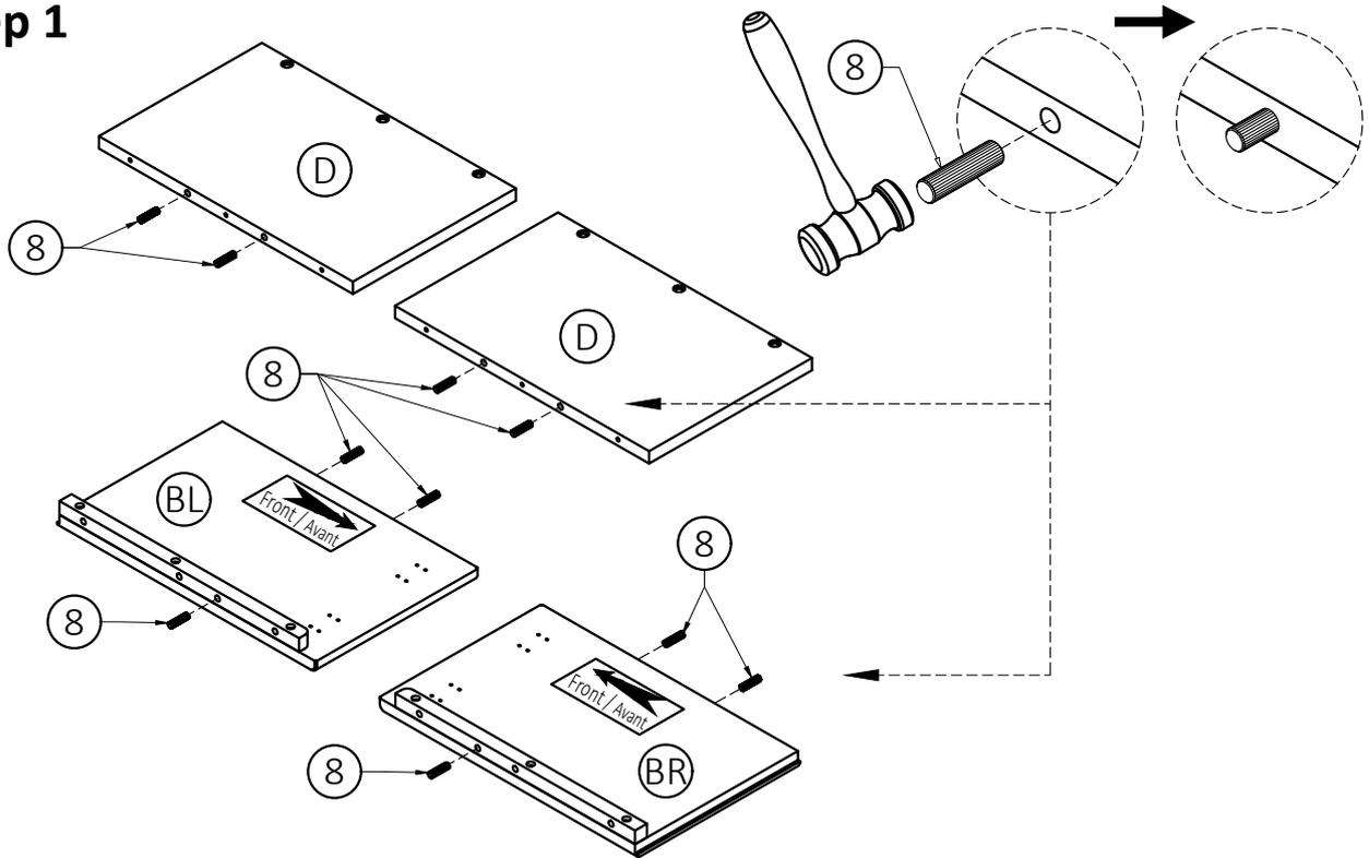
1. Insert Dowels (8) into guide holes on Dividers (D) and Sides (BL, BR).
