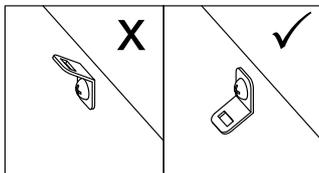
3. Drill a 3/16 inch hole in the wall. Press the plastic anchor into the hole and gently tap until the flange on the anchor is against the wall surface.
