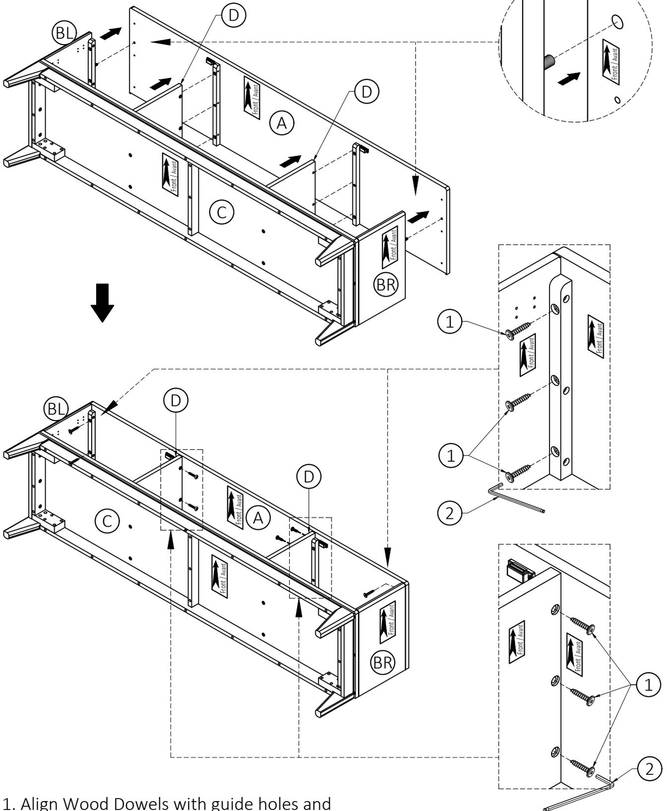
1. Align Wood Dowels with guide holes and attach Sides (BL), (BR) and Dividers (D) to Top (A).
