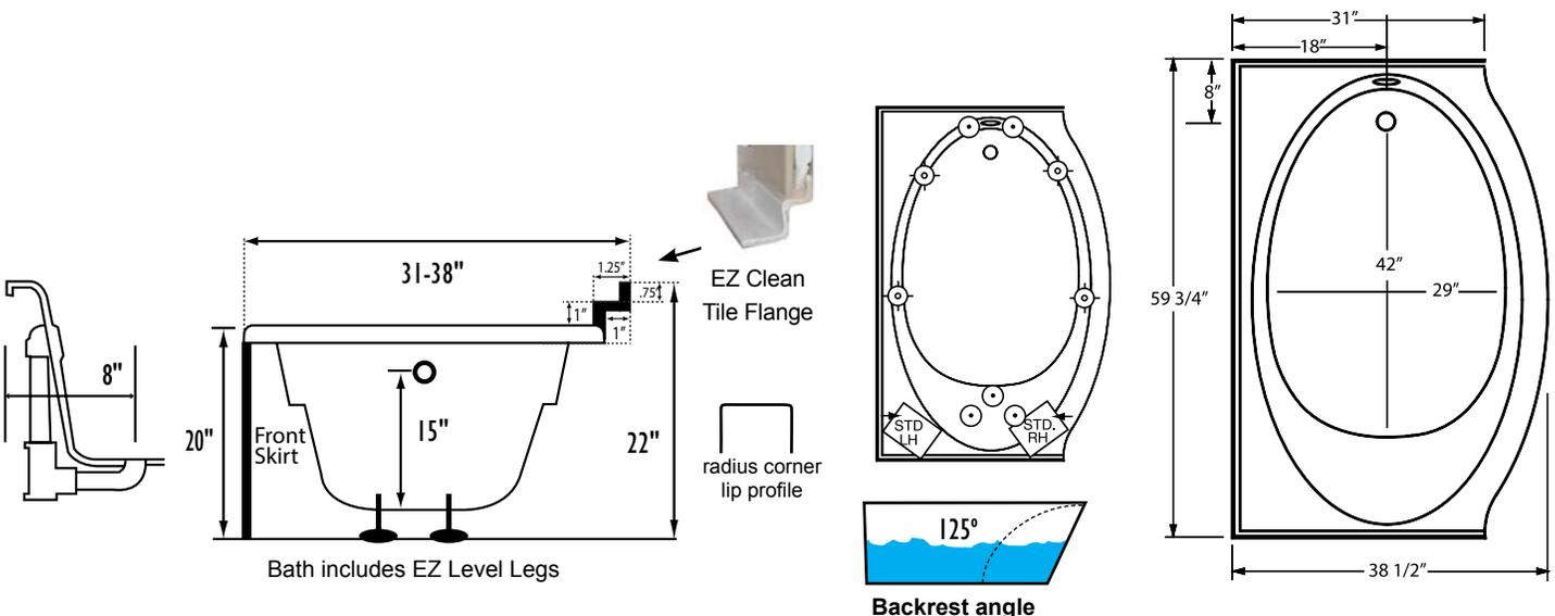
Some standard & most alternate pump locations may stickout past perimeter of the bath 1"-3". NOTE: Graphics may not be to scale. Specifications and features are subject to change without notice and are ± .25". All final measurements should be taken from tub on site. Access 18"x 18" or larger is required for each pump. Consult your contractor for installation requirements.
