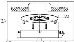
Step.2:Remove mounting bracket (A) from fixture and install to electrical box.
