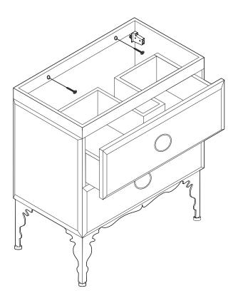
2 Apply a bead of silicone on the top of the cabinet and place the countertop on to the cabinet. Apply a bead of silicone on to the bottom of the sink and place the sink on the countertop.
