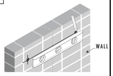
Once position is marked, drill 2 holes and insert anchors if stud is not available
