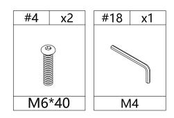
Use bolt #4 to attach preassemble leg(M) to bottom panel (B),make sure all holes aligned and tighten bolt #4 with allen key#18.
