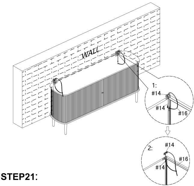
3. Let the plastic belt #16 pass through bracket #14 and pull tightly
