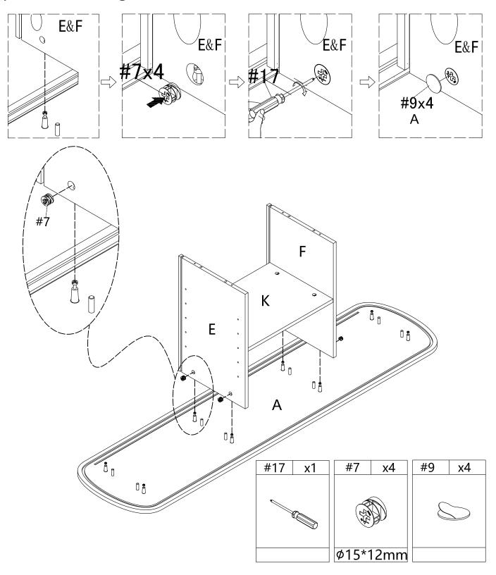
Insert side panel D)&(G) into the corresponding hole of top panel (A), and then insert cam bolt #7 into the corresponding hole of panel(D)&(G), tighten cam bolt #7 with screwdriver#17.
