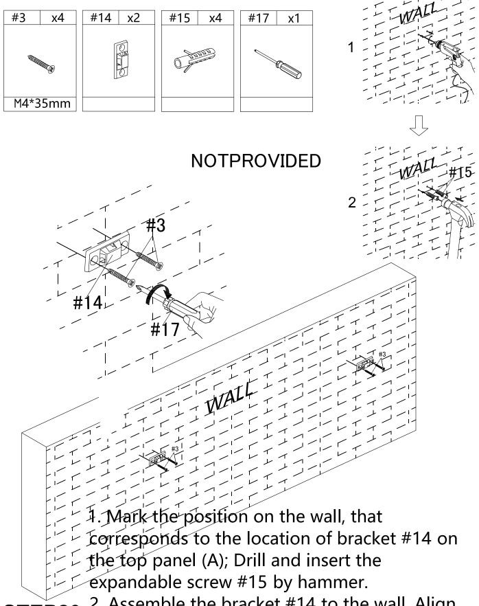
STEP20: 2. Assemble the bracket #14 to the wall. Align the hole in the bracket #14 with the expandable screw #15, use screw #7 to attach it, tighten screw #7 with screwdriver #17.
