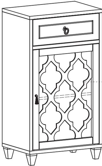
To move door up or down, loosen screws as shown and move door to suit. Re-tighten screws.
