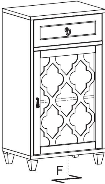
To move door left or right, loosen screw as shown and move door to suit. Re-tighten screw.
