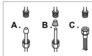
Connect to water supply lines with either:
