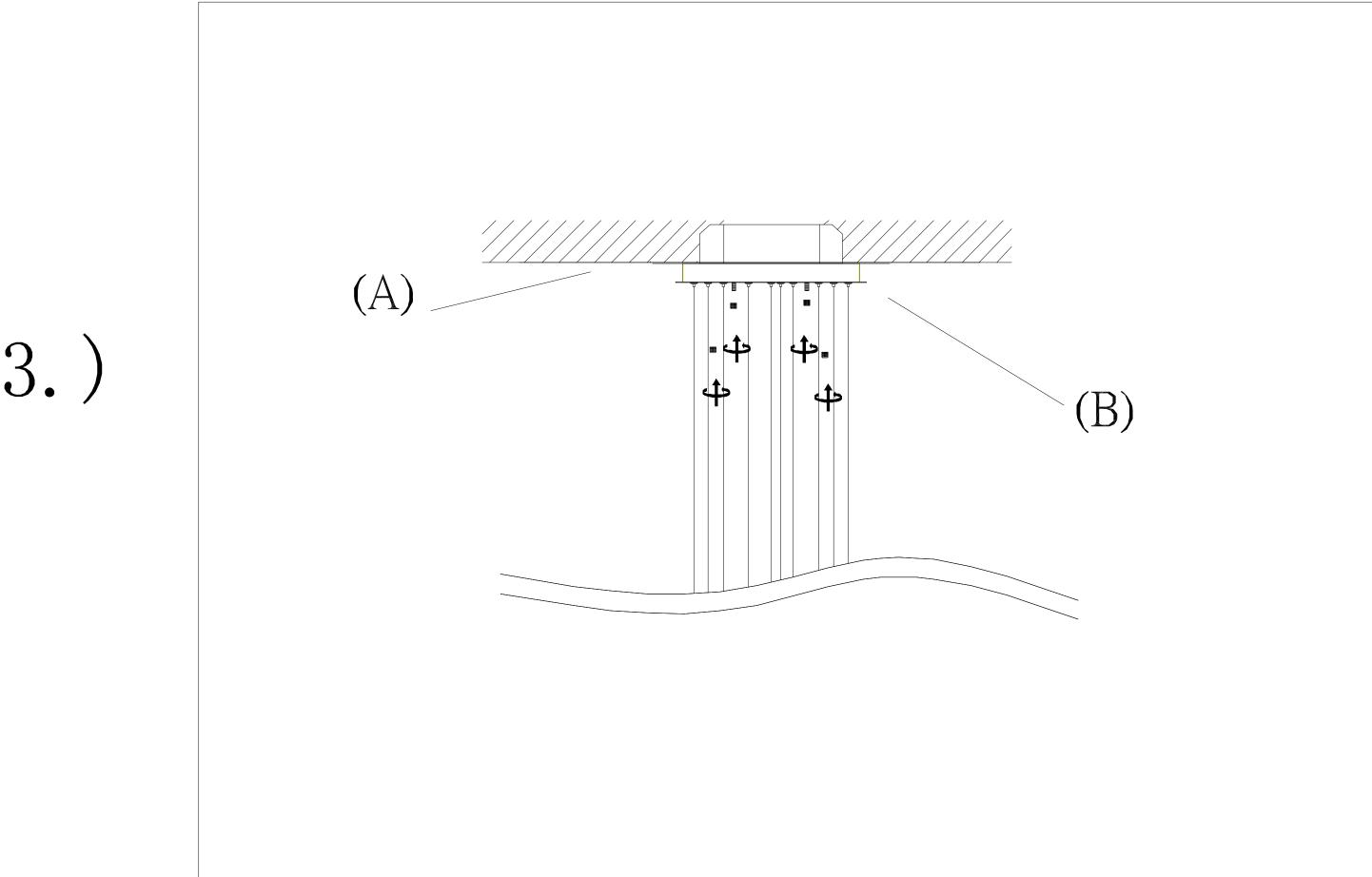
Step 3:Install Body (B) to Mounting Bracket (A) and tighten screws on the sides of the canopy to secure
