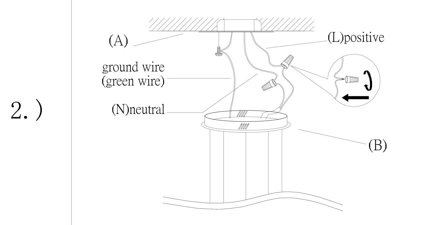
Step 2: Use push pins to adjust wires to desired mounting height. Wire fixture to wires in outlet box. See dual plastic wire instructions for more details. Install Green wire to Ground Screw.
