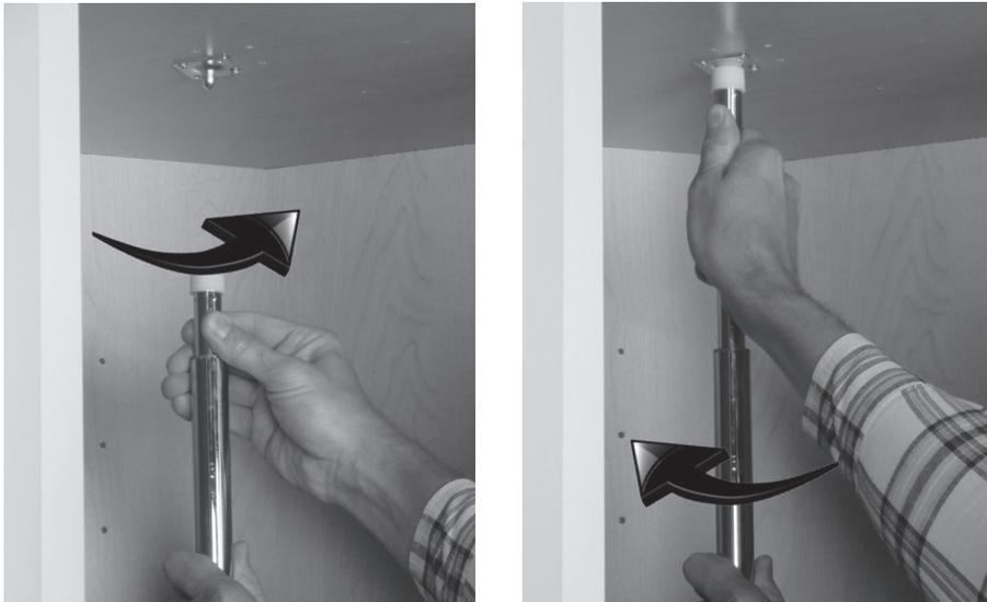
Holding onto the lower pole, twist the upper pole counter-clockwise to release. Extend pole upwards until it rests firmly against the Top Mounting Support and tighten by turning the upper pole clockwise.
