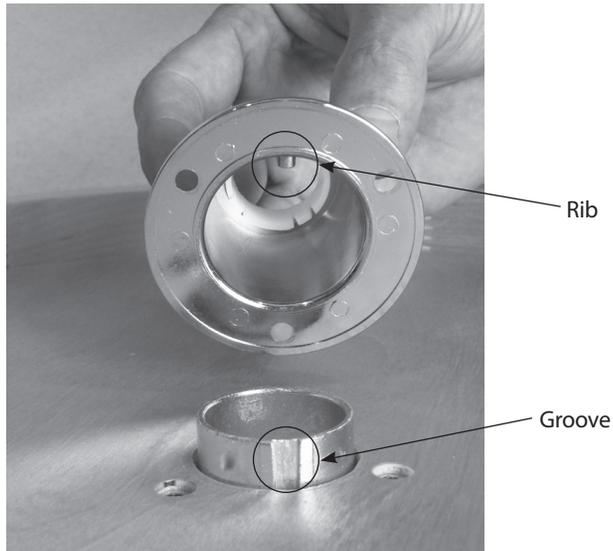
Insert one Shelf Hub through the bottom of a shelf as shown. Place one Shelf Hub Cone on the top of the shelf and fasten using (3) #8 x 1/2" Flat Head Machine Screws provided. NOTE: Make sure the rib inside the Shelf Hub Cone is aligned with the groove in the hub (see picture). Repeat with second shelf.
