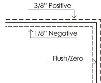
Use scissors to cut along the line of the paper template for you desired reveal type (Negative, Positive or Flush Reveal)
