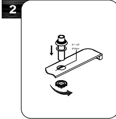
Insert body assembly through selected hole in sink. Secure body to sink by screwing the mounting nut from the underside of the sink. Hand tighten only.
