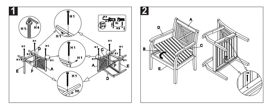
Step 1: attach right side (D) to the back (A). Then attach support L (E) and support S (F) to the right side (C) as shown on the picture by using the Allen Bolt (H1) and tighten with the Allen Key (H4). Continue with the left side (C) in the same way. Make sure to tighten all bolts (H1) before you continue with step 2.
