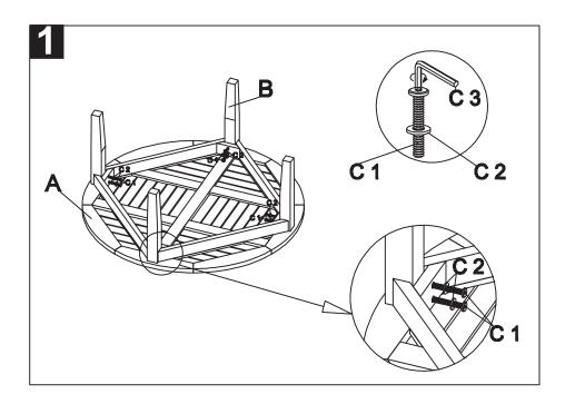
Step 1: attach the leg (B) to the top (A) by using washer (C2) and Allen Bolt (C1) as shown on the picture. Tighten all legs by using the Allen Key (C3).
