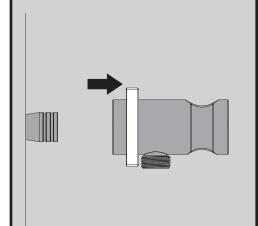
Slide Supply Elbow over the Pipe Adapter. Center the Outlet port on the wall. Outlet port should be pointing downward when complete. Tighten Set Screws (both top and bottom) with 2mm Hex Key Wrench included.
