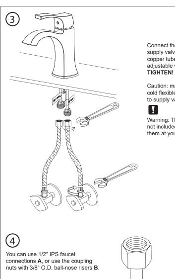
Connect the flexible hoses to water supply valves (not included) and copper tubes, and tighten it with adjustable wrench. **DON'T OVER**
