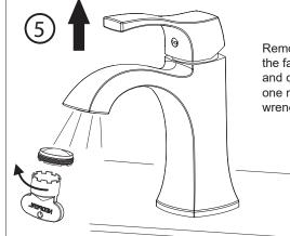
Remove the aerator by aerator wrench. Turn the faucet handle all the way on, turn on hot and cold water supply and flush water lines for one minute. Reinstall aerator by aerator wrench.
