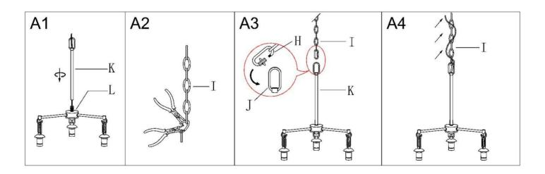
Step A1 » Screw stem (K) onto the top of arm assembly (L).
